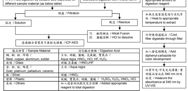
Note\*\*: (1) 針對非金屬材料加入鹼性消化液,加熱至 90~95℃萃取. / For non-metallic material, add alkaline digestion reagent and heat to 90~95℃.
